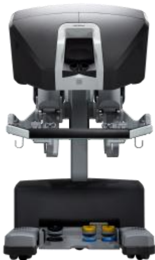
Figure 1. The working console on which one can notice the three subcomponents from top to bottom: video playback system, master control, crank
